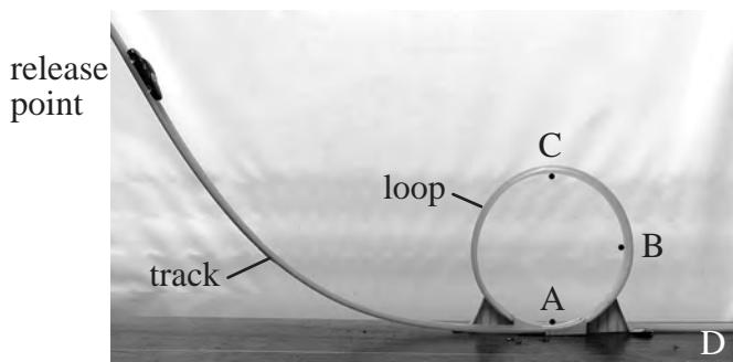
If the release point of the car is high enough, the car moves fast enough to pass point C and complete the loop, continuing to the end of the track at point D.
