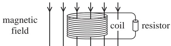
The magnetic flux density of the field through the coil is increased steadily from zero to a maximum value.
