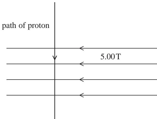
A force of  $1.20 \times 10^{-11}$  N is exerted on the proton.
