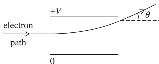
The electron is deviated through an angle  $\theta$ .
