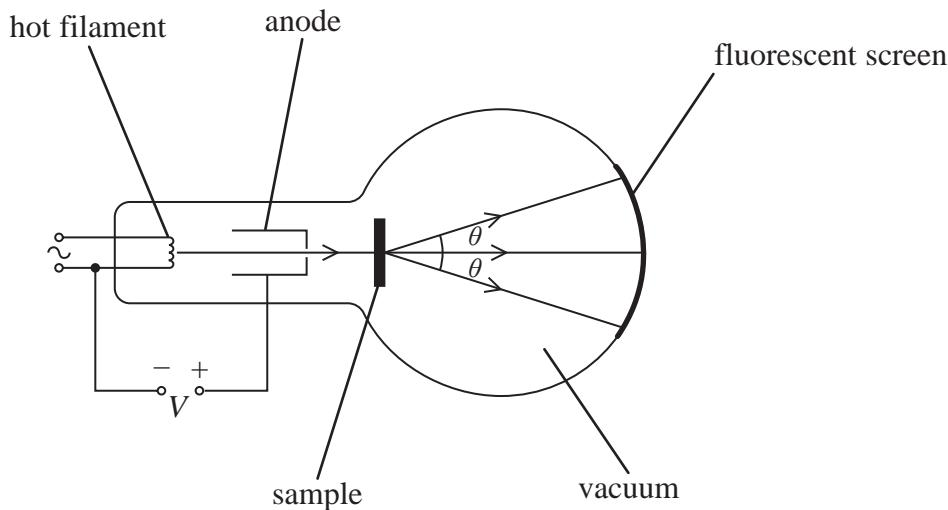
A beam of electrons is directed at a sample of crystalline material.
